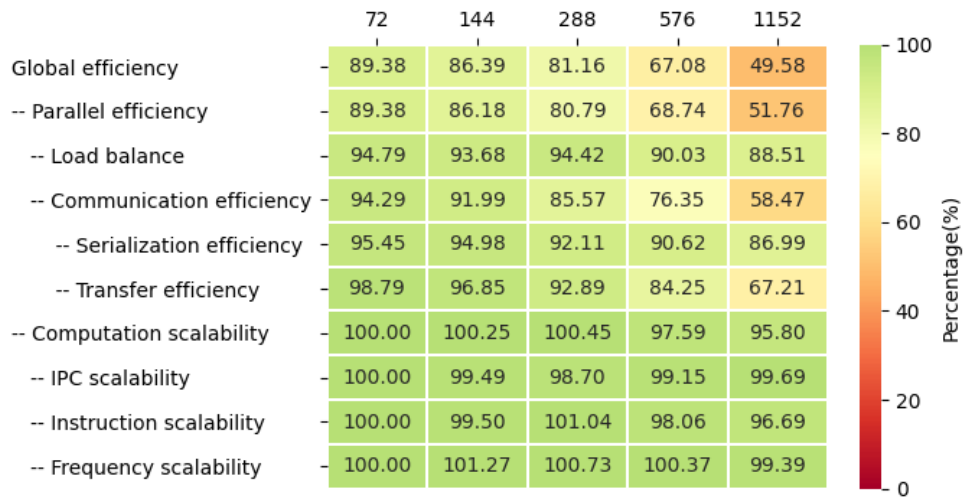
Figure 27: LaBS Turbulent Channel Iterative phase: Efficiency metrics.
