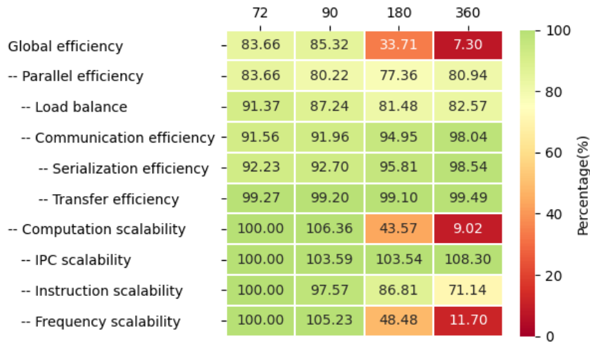
Figure 7: WaLBerla Turbulent Channel Initialization phase: Efficiency metrics.
