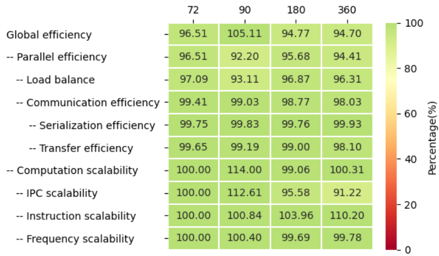
Figure 9: WaLBerla Turbulent Channel Iterative phase: Efficiency metrics.
