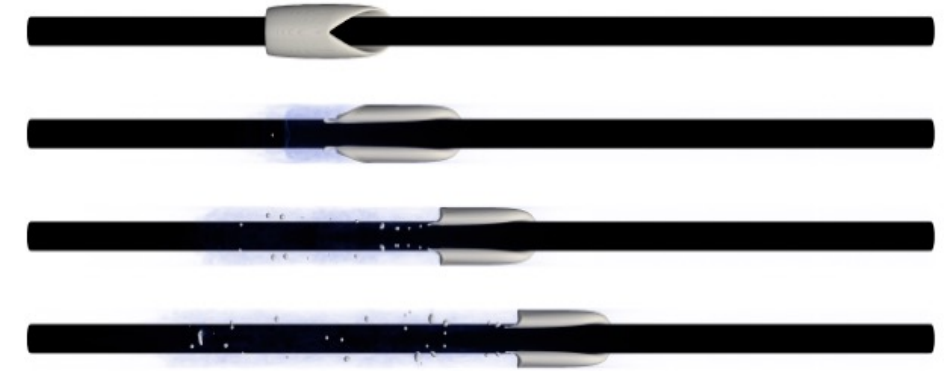
An example of the bubble propagation through the concentric annular pipe at different timesteps. 2
