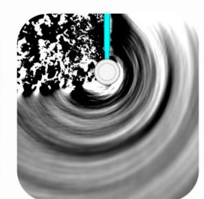
SCALABLE has chosen a suite of test cases reflecting the interest of the industrial partners. One of these test cases is the Lagoon landing gear. During the landing phase of an aircraft, the landing gear is an important source of noise and produces a non-trivial turbulent flow as illustrated by the visualizations of turbulence patterns and acoustic waves on the left.
