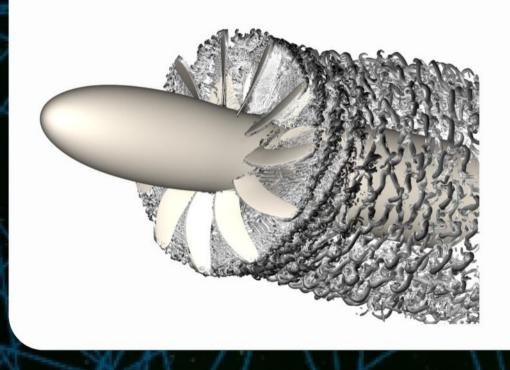
As a final application, SCALABLE is focusing on a novel contrarotating open-rotor propulsion system. This concept is one of the possible designs being studied to reduce emissions and improve efficiency in a post-carbon aviation future. The advancements from SCALABLE will be used to perform the LBM simulation of the Contra rotative open rotor Z08-AIPX7 case.
